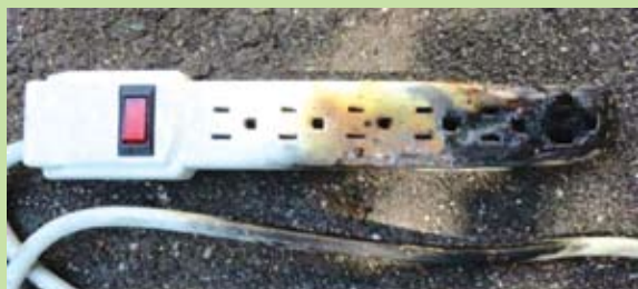
Result of a powerstrip being overloaded
